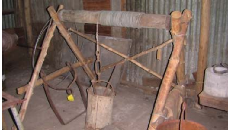
Windlass and bucket. A windlass was used to raise material from a mine shaft.
