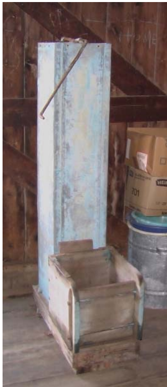
Windlass and bucket. A windlass was used to raise material from a mine shaft.
